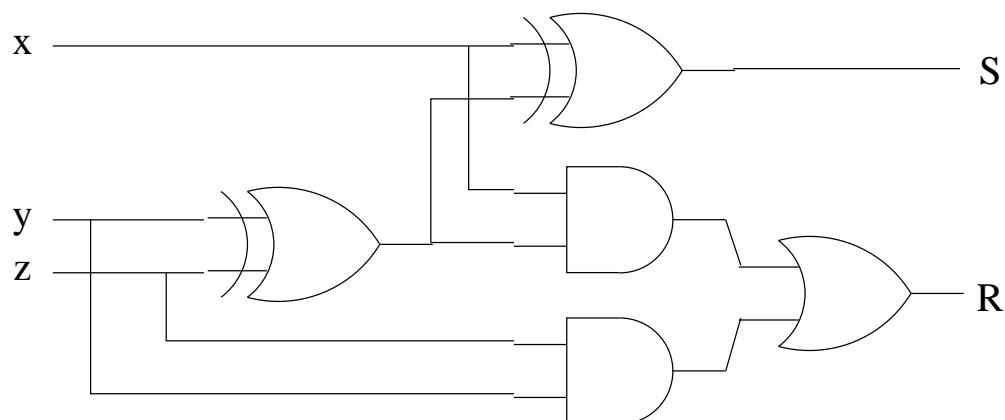
$$f(x, y, z) = (S, R) = (x \oplus y \oplus z, x(y \oplus z) + yz)$$
