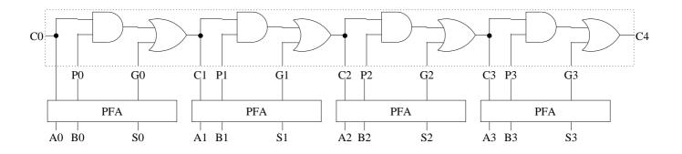
A solution to BRCA problem is to replace the RCP by a two-level circuit (2 gate delays)
