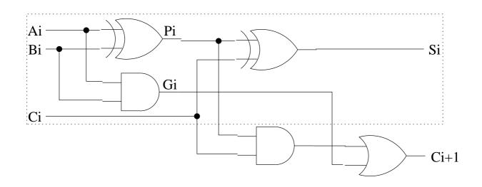
So for a 4-bit BRCA we have 8 gate delays in the RCP
